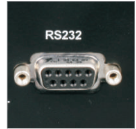
RS232 Port (Meter Interface)
